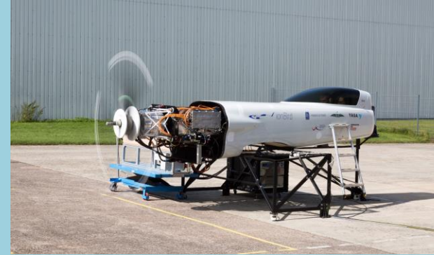
Full electric propeller test Source: Rolls-Royce
